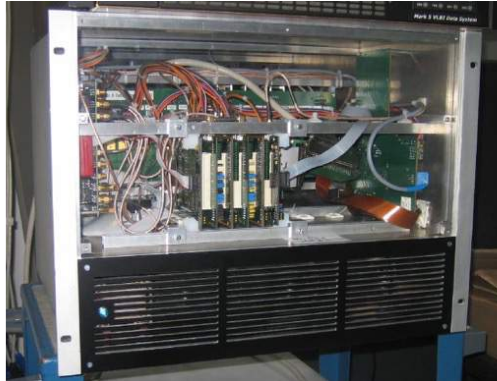
DBBC3 CORE3H processing board
